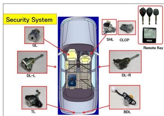
Figure 1. Auto-close System (Security System)
